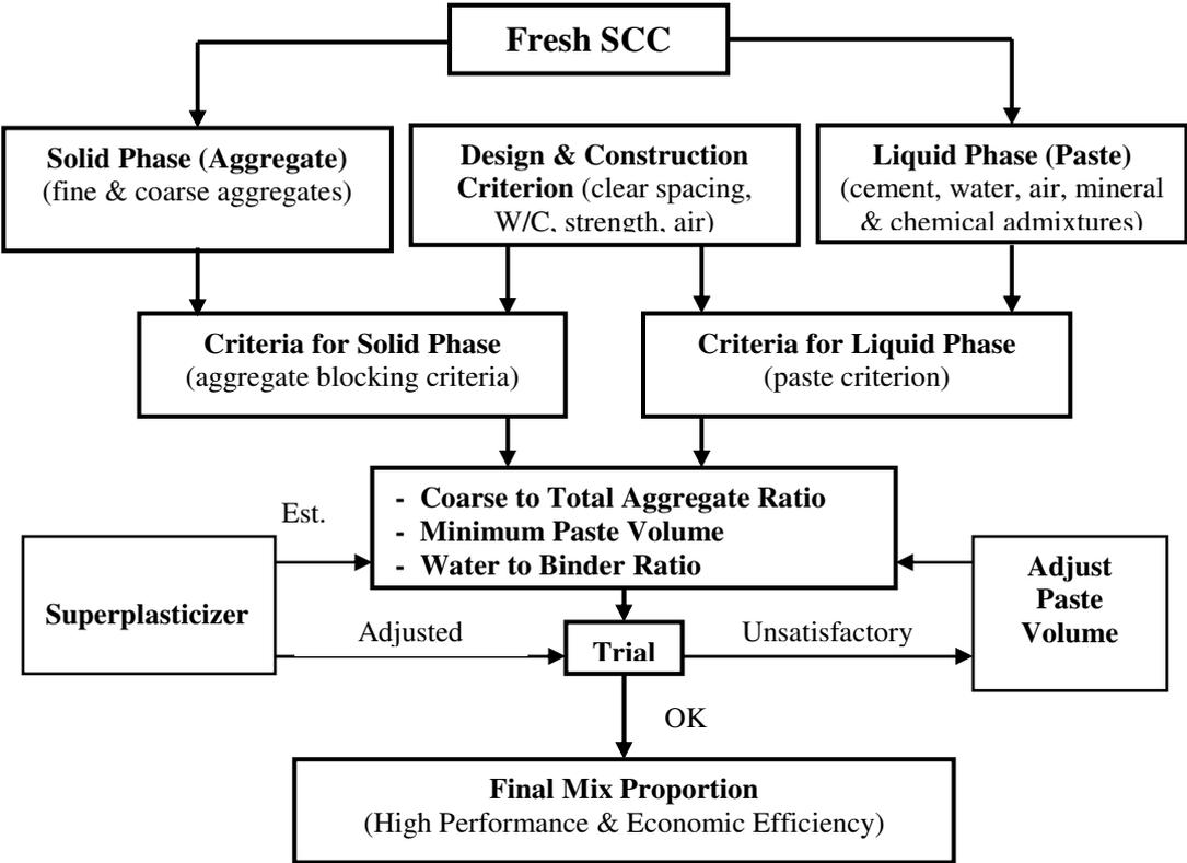
Fig. 1 Mix Design Procedure Flow Chart
