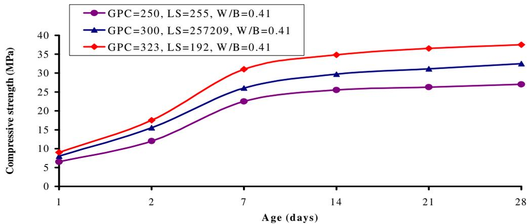
**Fig. 6: Compressive Strength of SCC Containing Milled Limestone and Different Cement Contents**
