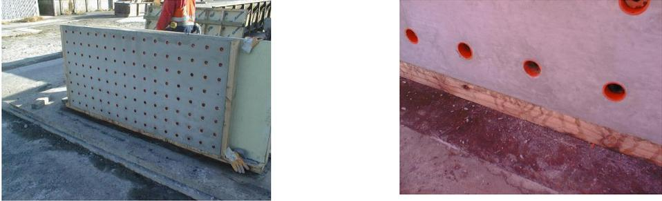
**Fig. 10: Arrangement of Plastic Ducts and Form Finish of UW Filters Plank**
