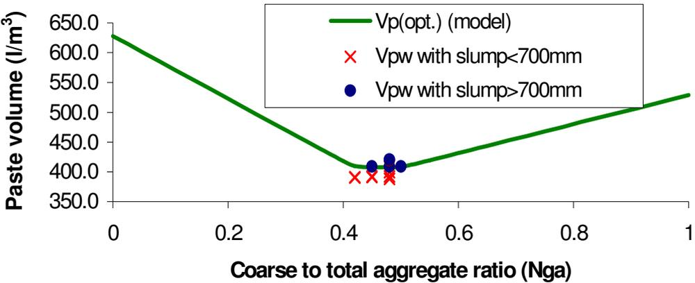
**Fig. 3: Minimum Computed and Tested Paste Volumes and Different Coarse to Total Aggregate Ratios**
