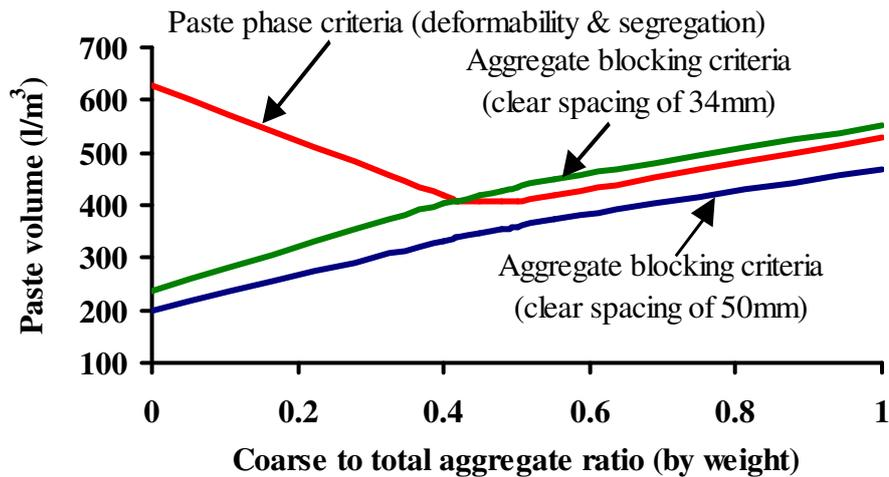
**Fig. 2: Typical Minimum Required Paste Volumes Computed from Aggregate Blocking and Paste Phase Criteria.**
