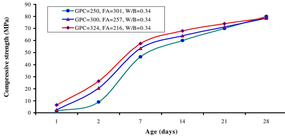
**Fig. 5: Compressive Strength of SCC Containing Fly Ash and Different Cement Contents**
